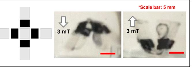
swimmer robot by using NdFeB and Fe<sub>3</sub>O<sub>4</sub> microparticles respectively and checked its motion. We mimicked the swimming method of the frog to actualize the swimming motion in the fluid.
