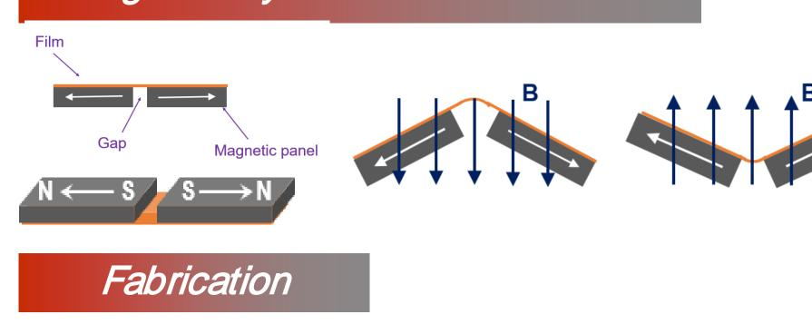
The basic method used in this technology is the magnetically actuation mechanism. It utilizes the basic characteristic of the magnetized materials to align in a specific direction according to **their magnetization** direction under the external magnetic field.
