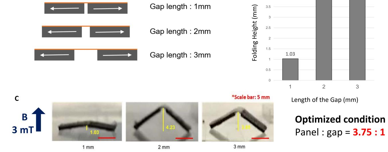
Fig. 4. A. B. C. The result shows that the robot shows the most activated movement with 2 mm gap. Therefore, the optimized length ratio between the panel and the gap was 3.75:1
