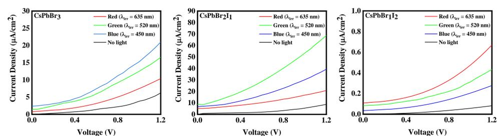
**Figure 4.** Current density-Voltage curve under Red(635nm), Green(520nm), Blue(450nm) radiations
