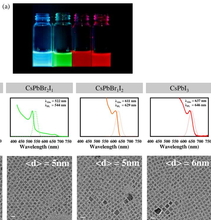
**Figure 1.** (a) Colloidal perovskite CsPbBr<sub>x</sub>I<sub>3-x</sub> QDs dispersions (in each vial, the QDs have a different halide composition) in hexane under an UV lamp ( $\lambda = 312\text{ nm}$ ) The image shows CsPbBr<sub>3</sub>, CsPbBr<sub>2</sub>I<sub>1</sub>, CsPbBr<sub>1</sub>I<sub>2</sub> and CsPbI<sub>3</sub> respectively. (b) Absorption (solid line) and PL spectra (dot line), (c) Transmission electron microscopy (TEM) images of CsPbBr<sub>x</sub>I<sub>3-x</sub> QDs.
