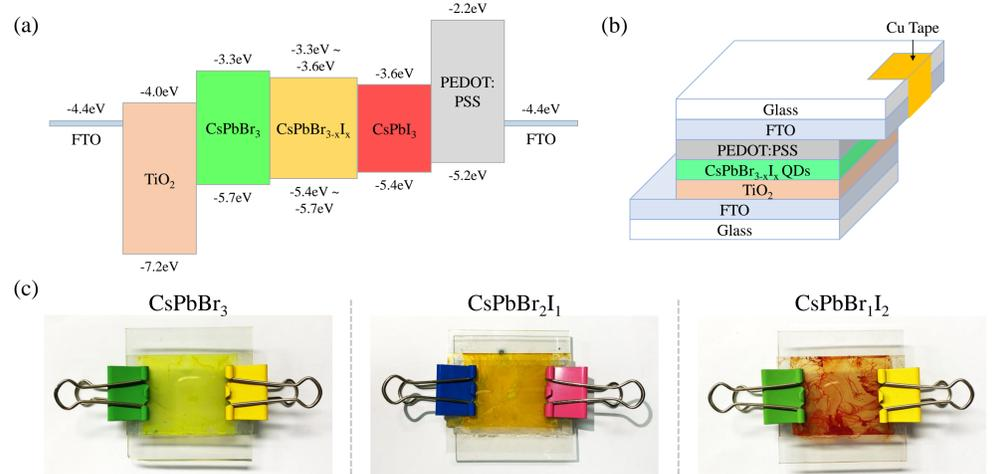
**Figure 3.** (a) Bandgap energy diagram of solar cell, (b) Structure of solar cell, (c) Photographs of three solar cell devices
