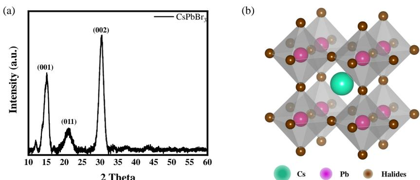
**Figure 2.** (a) X-ray diffraction (XRD) pattern of CsPbBr<sub>3</sub>, (b) Structure of CsPbX<sub>3</sub> (X = Cl, Br and I) Perovskite
