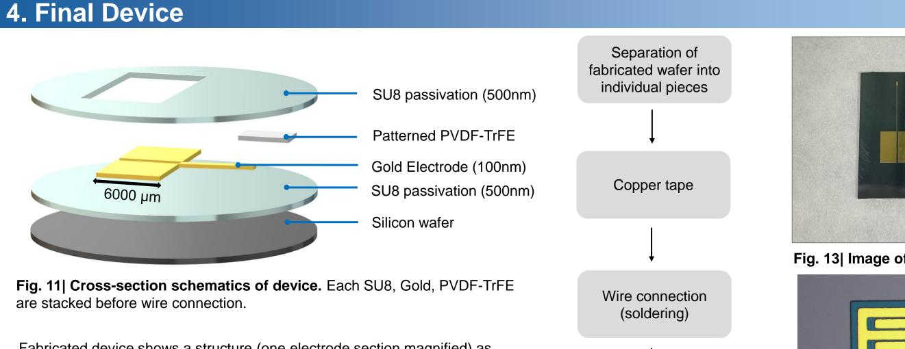
Fabricated device shows a structure (one electrode section magnified) as depicted in fig. 11. PVDF-TrFE is patterned directly onto the electrode for which it is the location to collect pressure stimulation. By consequently following additional steps in fig.12, the device can be characterized, connected to external examination devices. Device is shown in fig. 13, and fig. 14 shows the electrode section of the device. Thickness of electrode is 30 µm with separation distance of 10 µm.
