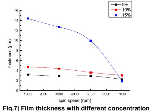
and spin coating rpm. Thickness decreases with increasing rpm and shows a drop around 5000 rpm. electrode and wire
