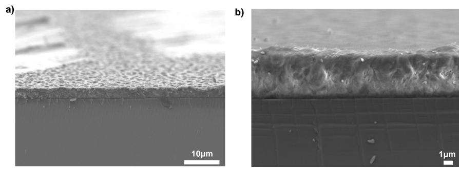
Fig.6| SEM of PVDF-TrFE film deposited on Silicon Wafer. Side view of sliced wafer coated with PVDF with each conditions of a) MEK 8% w/v
